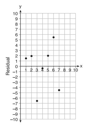
Based on the residual plot, the equation is a good fit for the data because the residual values are scattered without a pattern and are fairly evenly distributed above and below the *x*-axis.
